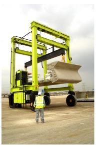
Right: With a light flexible structure and open cab, this low cost straddle is able to operate on good quality hardstand—a surfaced pavement is not required (Australia)
