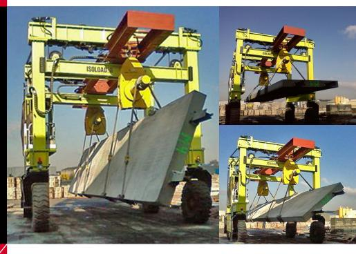
Straddle Carriers are not just for lifting heavy pre-cast concrete loads – they are cost effective solutions for handling lighter loads from 10 to 50 tonnes.
