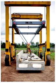
Above left: The lighter grade concrete pavement in this factory producing road and rail segments required a straddle that was small, light and cheap (Thailand).
